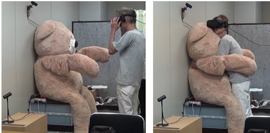
Fig. 1 MetaHug system: a robot hugs a participant wearing a HMD that shows a computer-graphics-based agent
