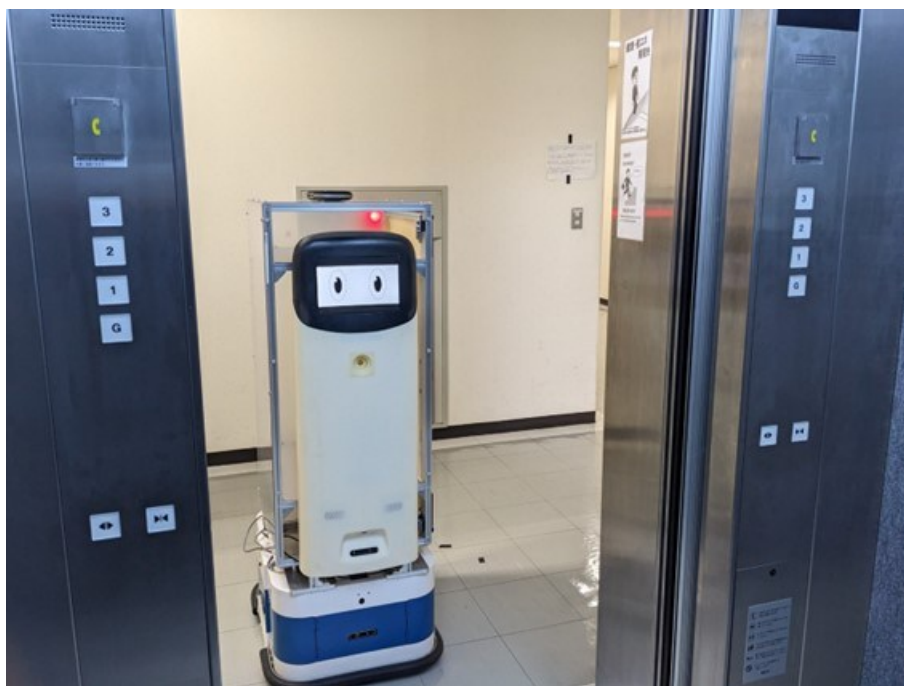
Fig. 1 Mobile robot takes a social elevator
